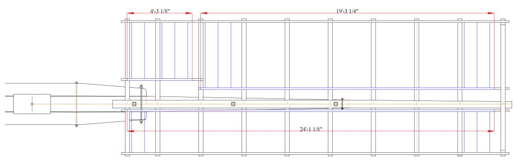
Shutter Pivot lines and Working Uplongs shown in blue
