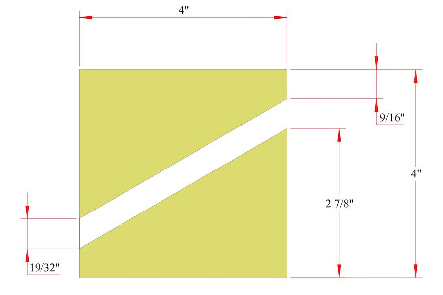
Slot in oak fan stock to suit 1/2" boards. Blade set at 30 deg. NB Fantail to rotate anti-clockwise
