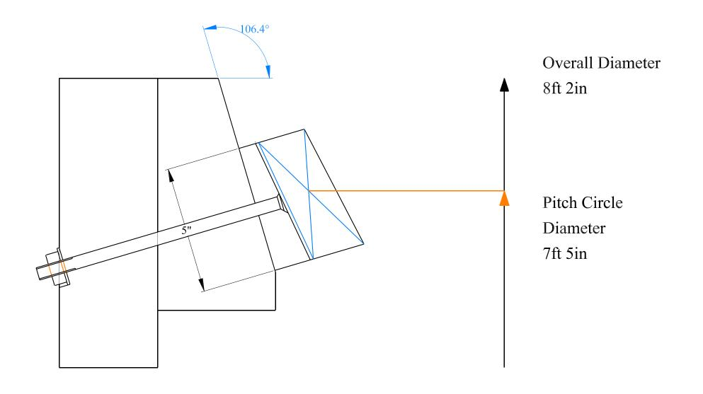
Fig 3.7 WICKEN WINDMILL: Section of rebuilt Brake Wheel Rim
