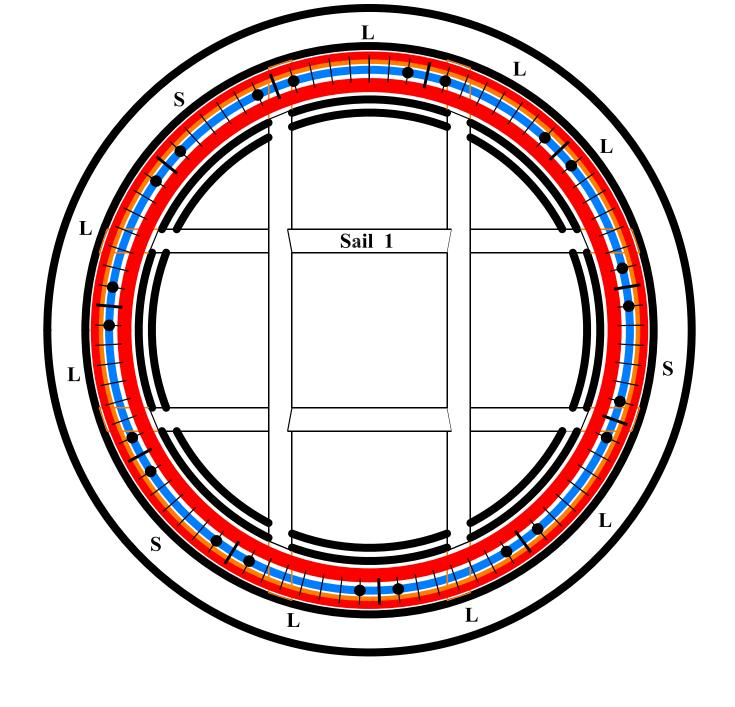
Fig 3.6 Wicken Windmill: Brake Wheel Layout (from rear)
