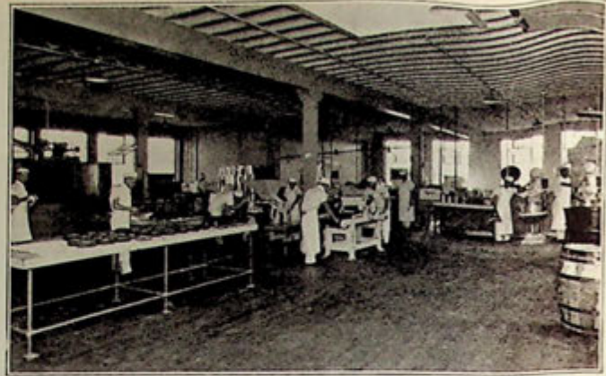
Davidson's Cake Shop, Portland, Oregon, is equipped with a Fish rotary oven, a Read cake mixer and flour sifter, a Koltzen cake depositor and a 15x30 ft ice box.
