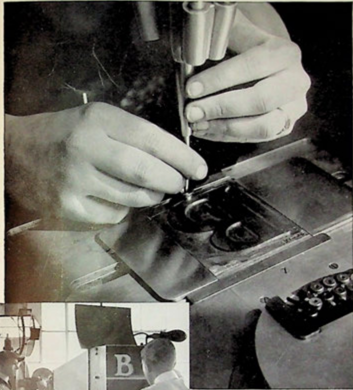
Checking the uniformity and accuracy of a newly-designed letter in the Projectoscope where an error of even a fraction of a thousandth of an inch is instantly apparent.
