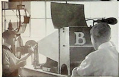
Checking the uniformity and accuracy of a newly-designed letter in the Projectoscope where an error of even a fraction of a thousandth of an inch is instantly apparent.
