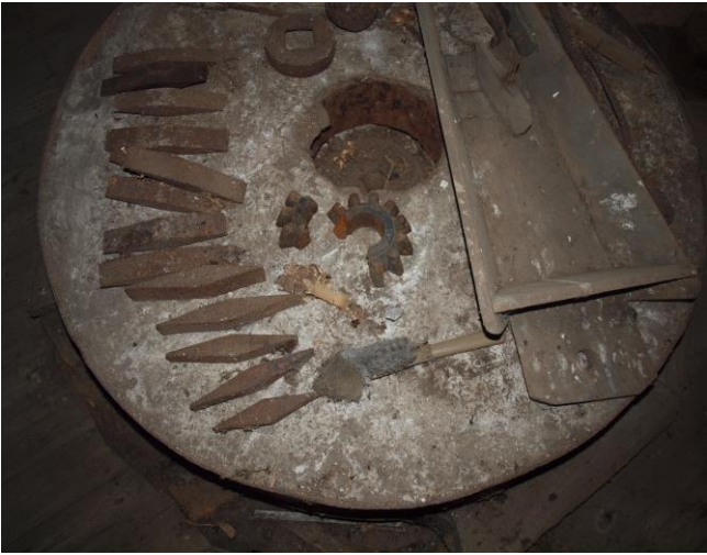
Fig.5 Miscellaneous items on one of the millstones, including the broken fantail pinion
