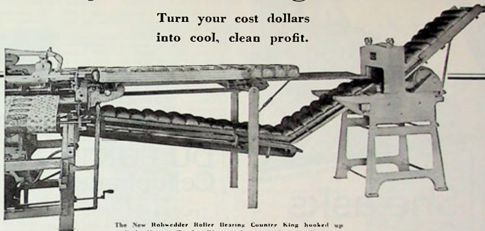
The New Rohwedder Roller Bearing Counter King hooked up with the Hayssen Trayless Wrapper forms an ideal One-Man unit.
