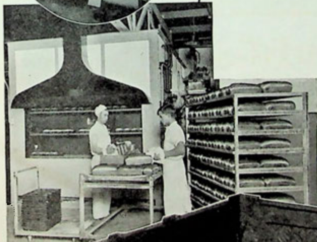
In Oval: Greater "punishment" can be given dough made with Russell-Miller high-gluten flours. At Left: Six hundred loaf traveling oven, gas fired—one of two in the new plant of the Barker Baking Co. The oven heats to baking temperature within 20 minutes of firing. Below: The new home of the Barker Baking Co., representing 10 years' growth from a three-man shop—concrete evidence that quality pays.
